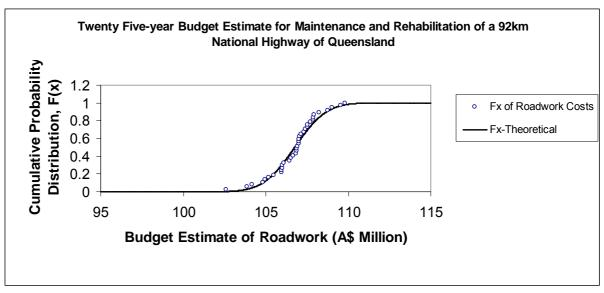
Figure 11 Cumulative distribution of budget/cost estimate for 25-year roadwork cost of a 92-kilometre National highway of Queensland (roadwork includes maintenance and rehabilitation)
