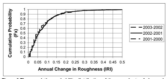
Figure 6 The cumulative probability distribution of the annual rate of change in road pavement roughness between the years 2002-03, 2001-02 and 2000-01
