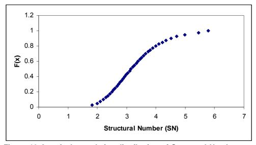
Figure 10 A typical cumulative distribution of Structural Number representing pavement strength sampled by Latin Hypercube Sampling Technique of one kilometre section for a 92-kilometre national highway
