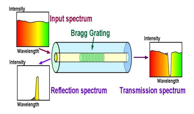
Figure 3. Fibre Bragg Grating
