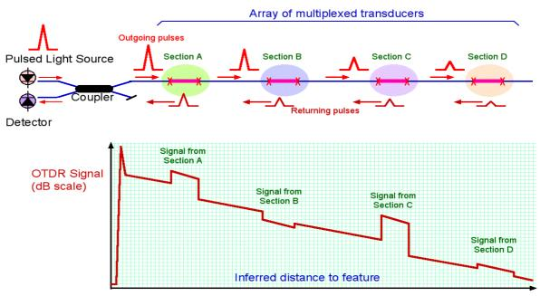
Optical Time Domain Reflectometry (OTDR) – Distributed Measurement.
