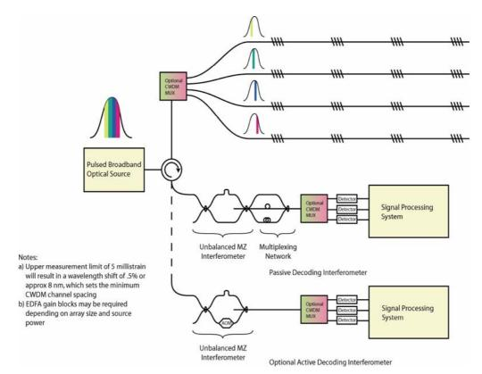
Figure 4. Point Array of Sensors
