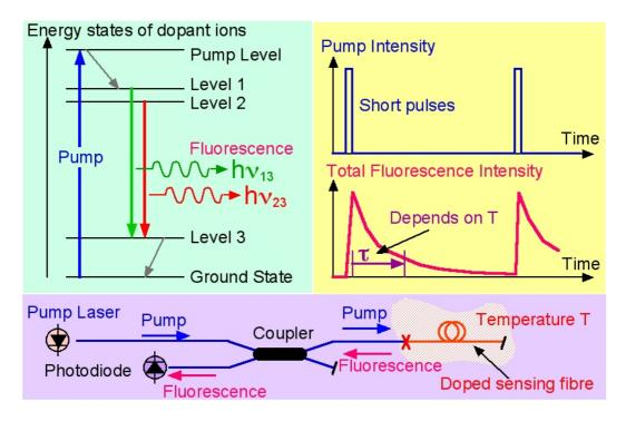
Figure 2. Fluoresence Decay Temperature Measurement.
