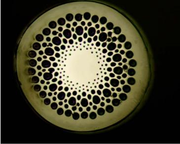
Figure 6. Holey Fibre
