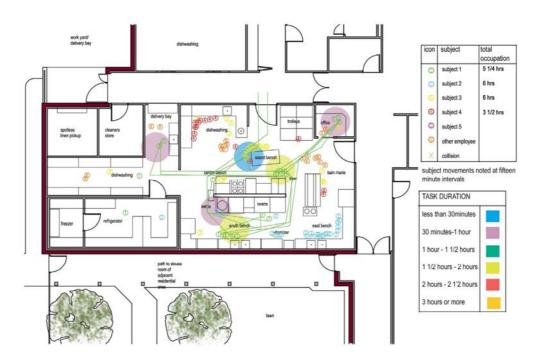
Figure 3: Mawson Lakes Kitchen Layout and Example Work Flow Pattern
