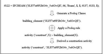
Figure 2: From an IFC building element to a job activity
