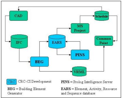
Figure 1: From 3D CAD to a construction schedule
