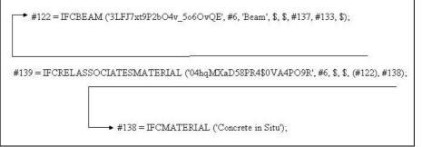
Figure 3: Inferring the construction method from IFC data
