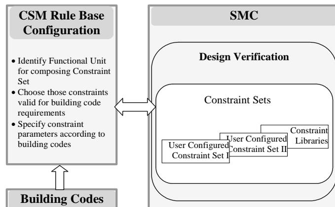
Figure 6. An illustration of developing CSM rule base for code checking.
