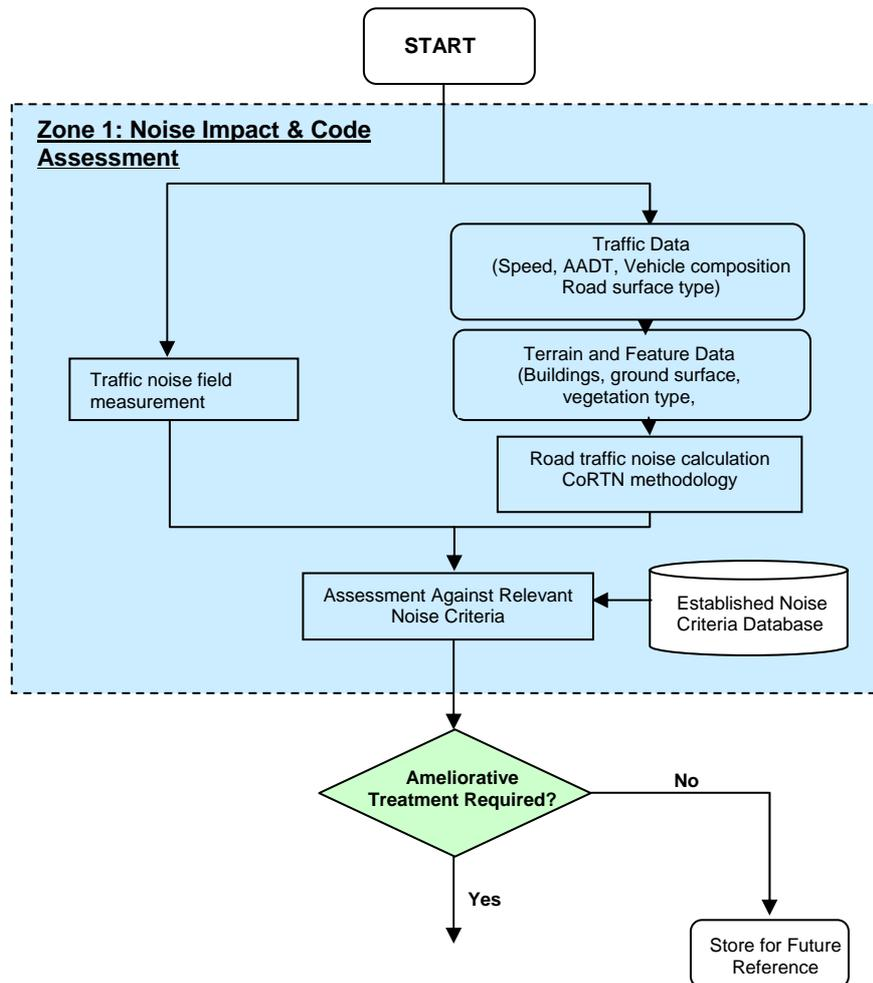
Figure 1 – Flow chart of the noise impact and code assessment zone
