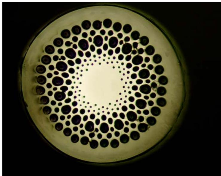
Figure 6. Holey Fibre
