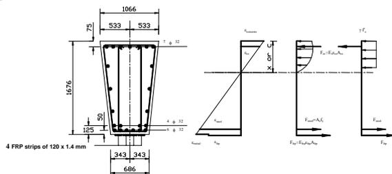
The section design for failure mode of yielding steel followed by concrete crushing
