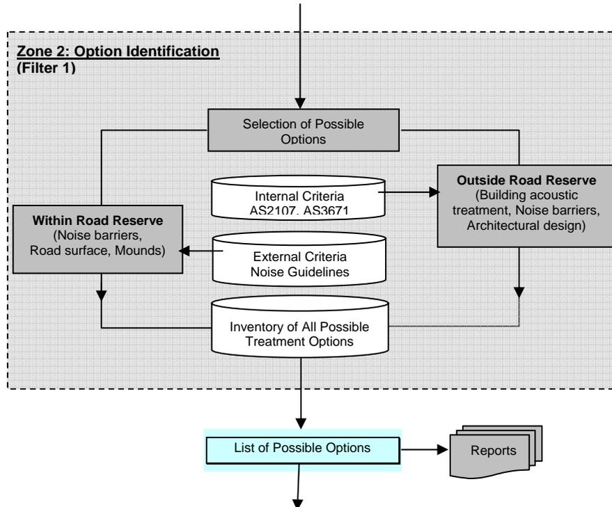
**Figure 2 – Flowchart of the option identification zone**
