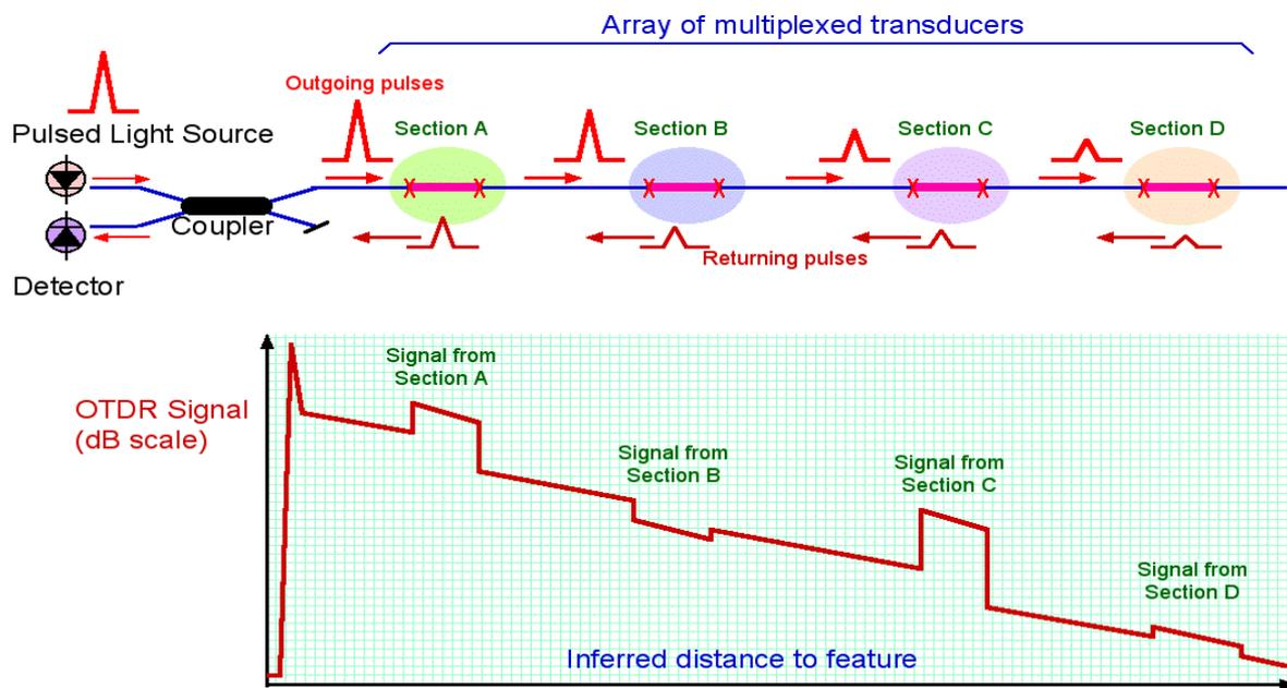
Optical Time Domain Reflectometry (OTDR) – Distributed Measurement.
