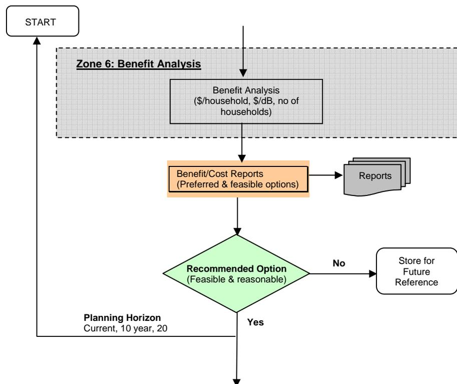
Figure 6 – Flowchart of the benefit analysis zone for different planning horizons
