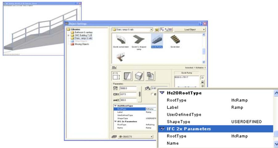
Figure 8. An example of converting an ArchiCAD object into an IFC object.
