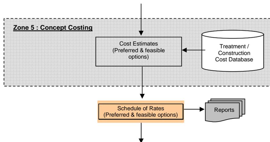
**Figure 5 – Flowchart of the concept costing zone**
