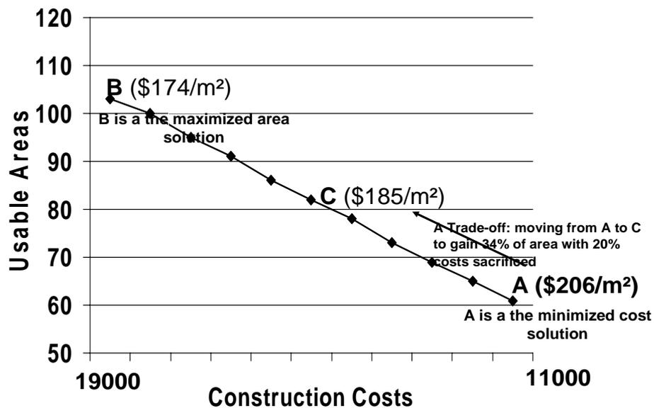
Figure 7. An example of design concepts for solving conflicting clients’ requirements (created from the data adapted from Balachandran (1988)).
