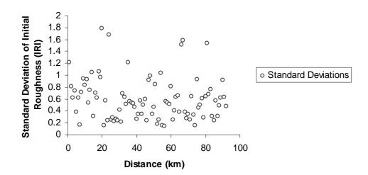
Figure 6. Standard deviation of initial roughness for each kilometre of a 92km national highway of Queensland
