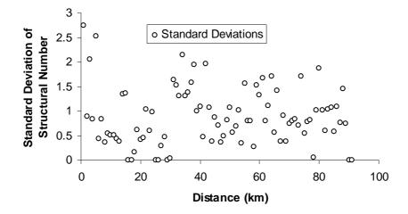
Figure 2. Standard deviations of the Structural Number for each kilometre of a 92km national highway of Queensland
