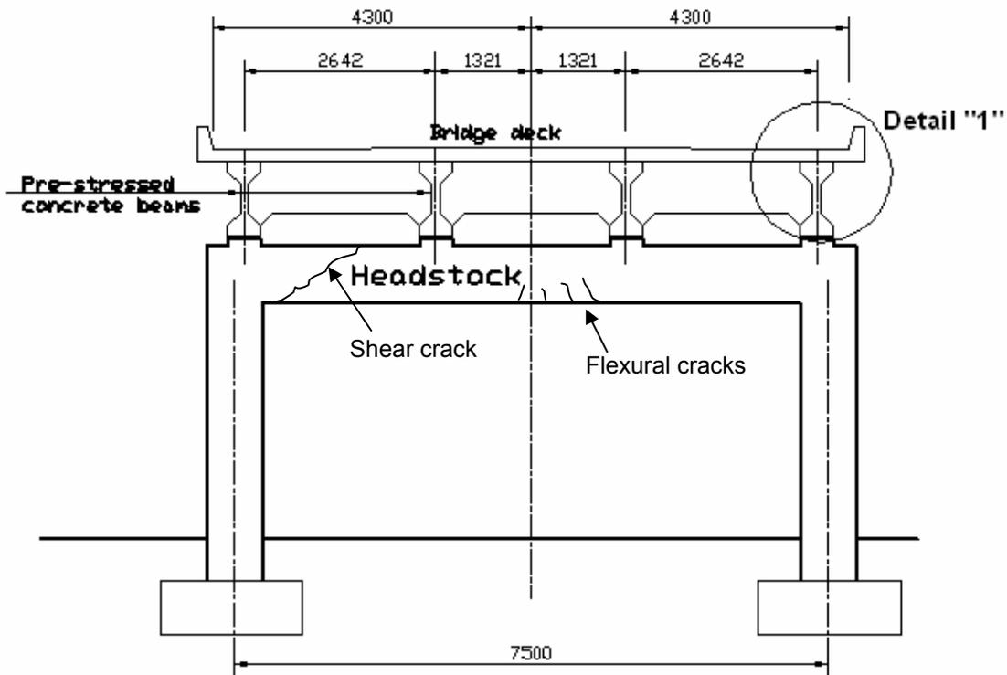
**Fig. 1 – A schematic elevation view of the headstock**
