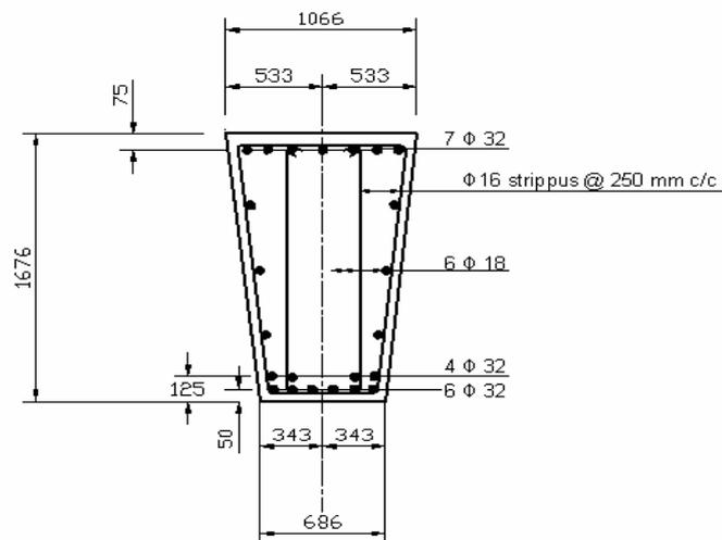
**Fig. 2 – Typical beam section of the headstock**
