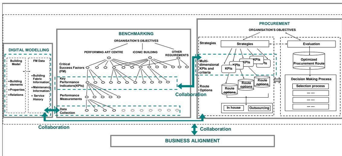
Figure 9. Illustration of a scenario of a future integrated FM system based on the integration of information resources.
