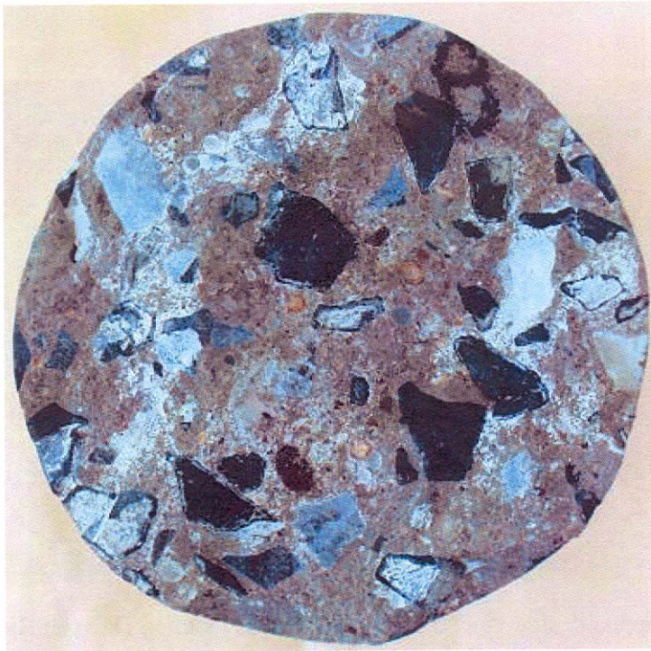
Photo 2. Concrete core sample from Dawson River Bridge (note the ettringite formations)
