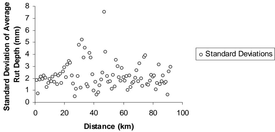
Figure 4. Standard deviations of average rut depth for each kilometre of a 92km national highway of Queensland
