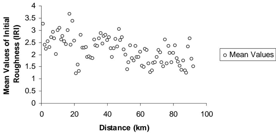
Figure 5. Mean values of initial roughness for each kilometre of a 92km national highway of Queensland
