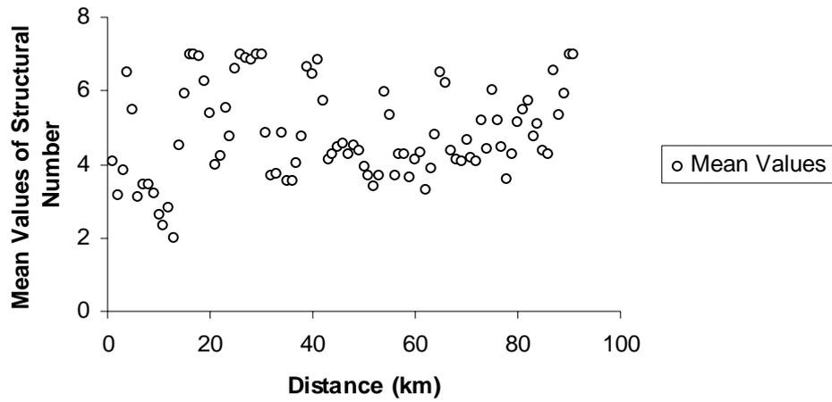
Figure 1. Mean values of the Structural Number for each kilometre of a 92km national highway of Queensland
