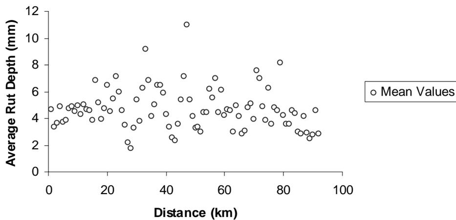
Figure 3. Mean values of average rut depth for each kilometre of a 92km national highway of Queensland.
