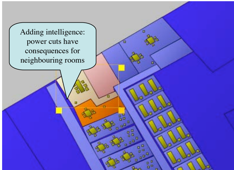
Figure 14: Computing and visualising the impact of taking a service out of commission
