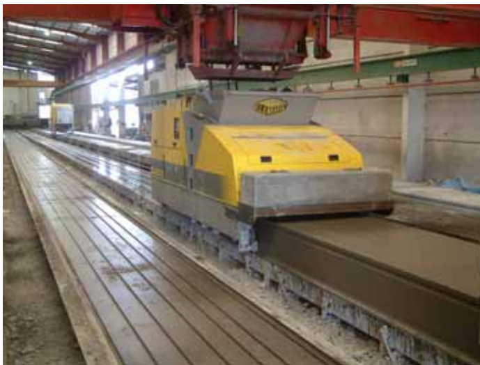
Figure 4.21: Hollowcore in production
