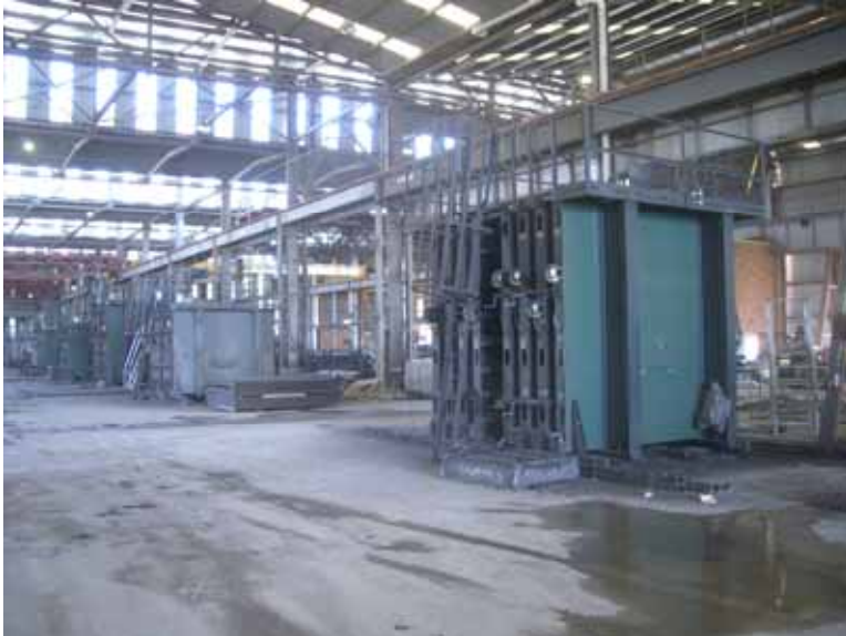
Figure 4.8: Vertical sound barrier moulds (Battery Moulds).
