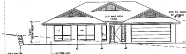
Case study 4 - brick veneer on slab, tiled roof, 194m 2 internal space with 4 bedrooms, 2 pedestals
