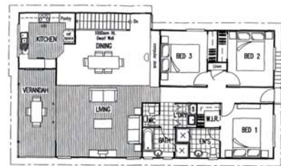
Case study 6 – elevated lightweight dwelling, metal roof, 189m internal space with 3 bedrooms, 2 pedestals. Elevations not provided
