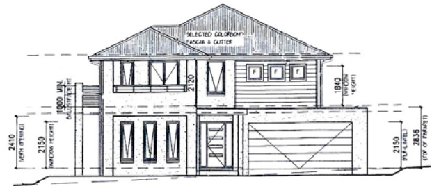
Case study 5 - two storey brick veneer on slab, metal roof, 287m 2 internal space with 4 bedrooms, 3 pedestals
