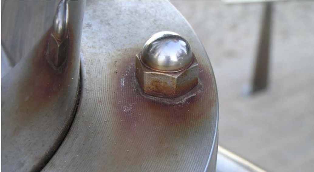
Figure 30. Red rust staining from bolt
