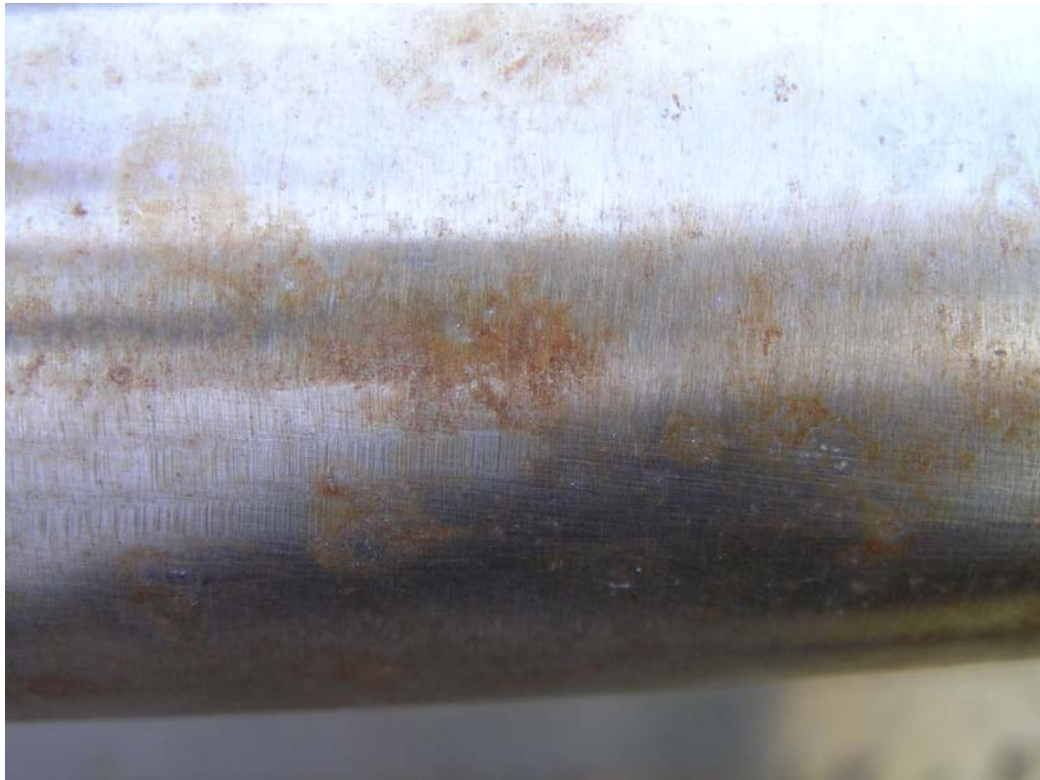
Figure 28. "Tea staining" on hand rail
