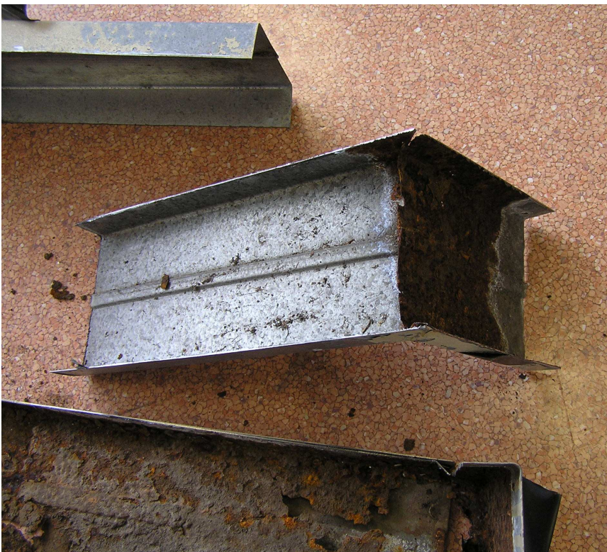
Figure A8, Top section insert showing no corrosion on the upper surfaces of the insert or the main part of the downpipe
