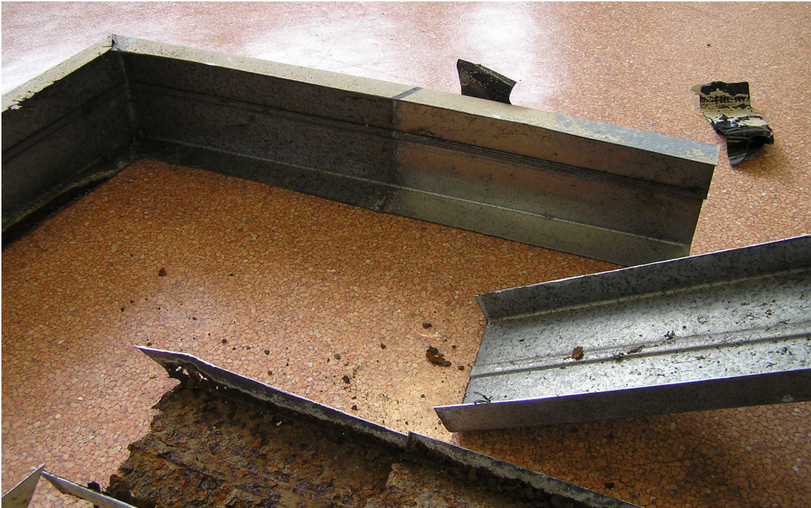
Figure A9, Top section insert showing no corrosion on the upper surfaces of the insert or the main part of the downpipe
