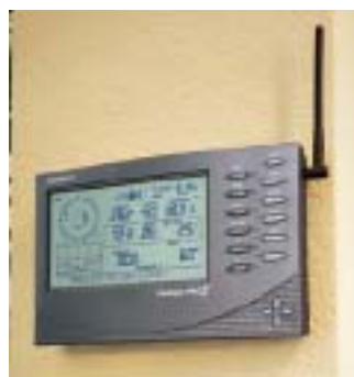
Figure 5-2 Monitoring system - internal console
