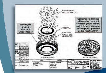
Exploded view of Ecoflex E-Pave Unit
