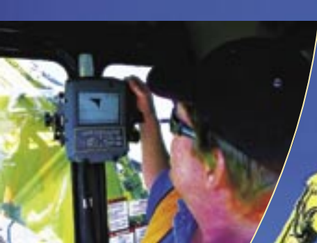
Using GPS to control machinery on the Port of Brisbane Motorway
