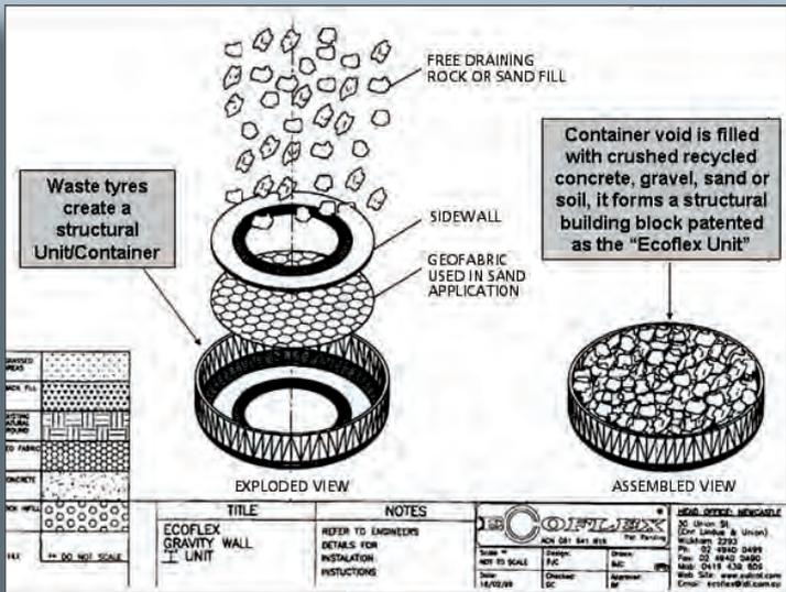
Exploded view of Ecoflex E-Pave Unit
