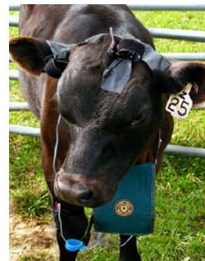
Figure 6. Bi-directional (mercury) motion sensors are attached to the calf's front legs, a gyroscopic sensor on the forehead and accelerometer on his right ear. The pouch hanging around his neck contains the radio frequency transmitter that sends the real time data to the (La Kitchen) Kroonde Gamma wireless UDP receiver [18]. It is connected by Ethernet to the computer running the data sonification with Max/MSP object-oriented programming environment.
