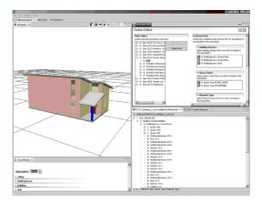
The "association" perspective is used to define the details of the relationships between a specification document and building model. This perspective allows the user to define which parts of the document are associated with which parts of the building model, and to visually inspect those relationships.
