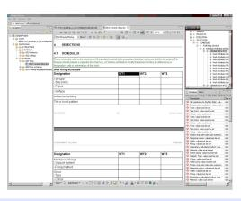
The "spec entry" perspective provides a default configuration of views and to inspect and edit the specification documents. It can embed Microsoft Word into the application for viewing and editing purposes, and provide an outline of the specification model
