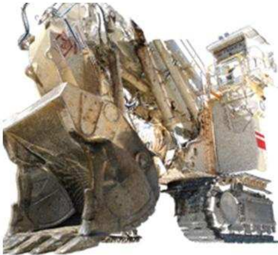
Figure 7.15 Laser scan of an excavator at Mt Keith mine. Colour has been applied to the point-cloud data points.
