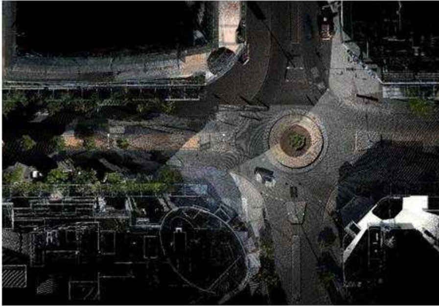
Figure 7.11 Plan view of the laser scan data of Grey Street, South Bank.
