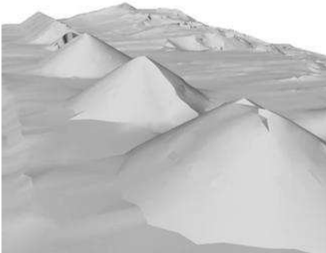
Figure 7.14 A surface model produced by laser scanning a mining pit at South Walker Creek Mine.
