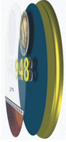
Figure 4.5 An 'exploded view' of BrailiantTouch® signage
